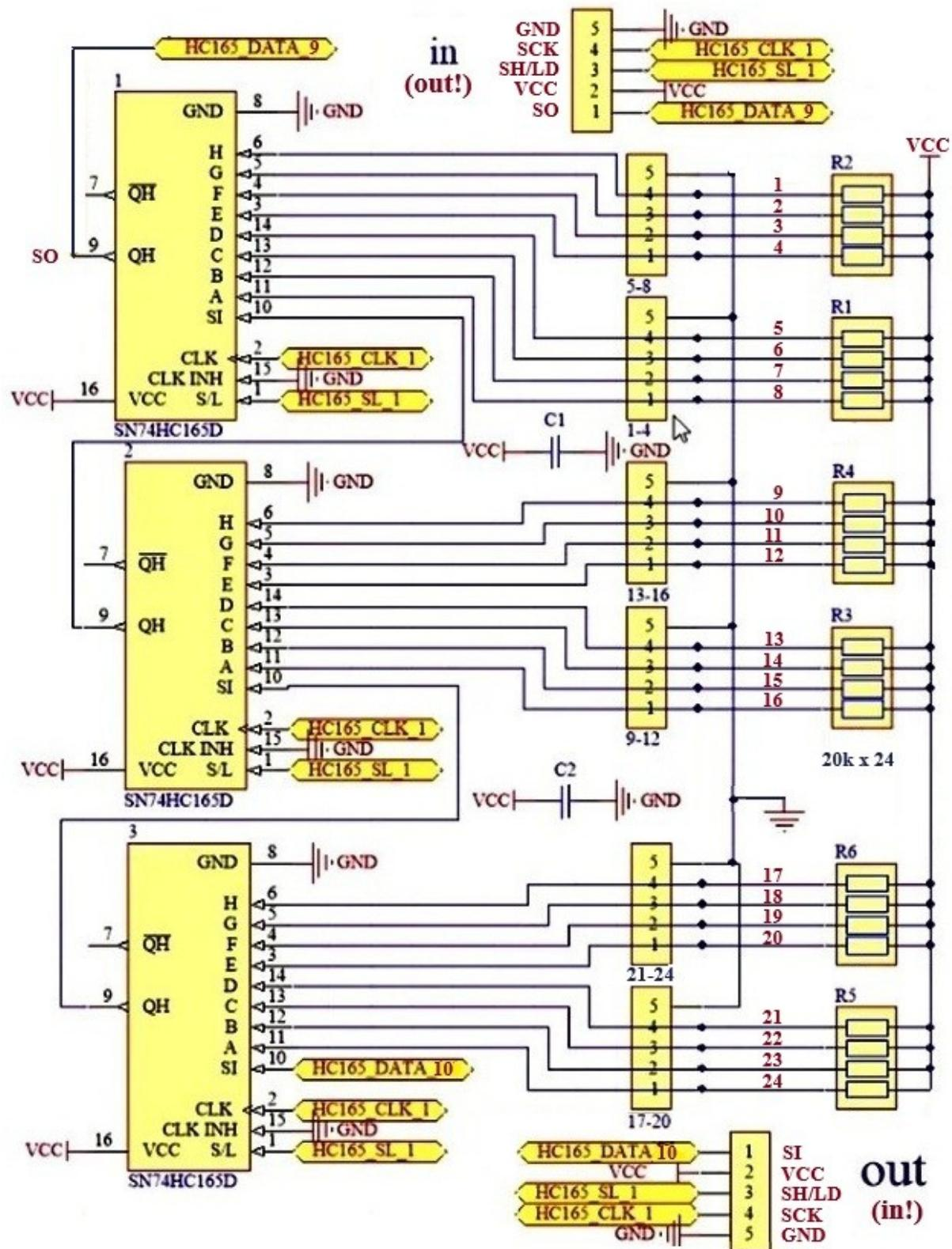
When the signal SH/LD is Low, parallel input data are loaded into the registers. When SH/LD is High, the data bits are shifted out serially via SO (= MISO). SH/LD must remain High during transfer of all 24 (or 25) bits. Refer to the 74HC165 data-sheet for further information.
