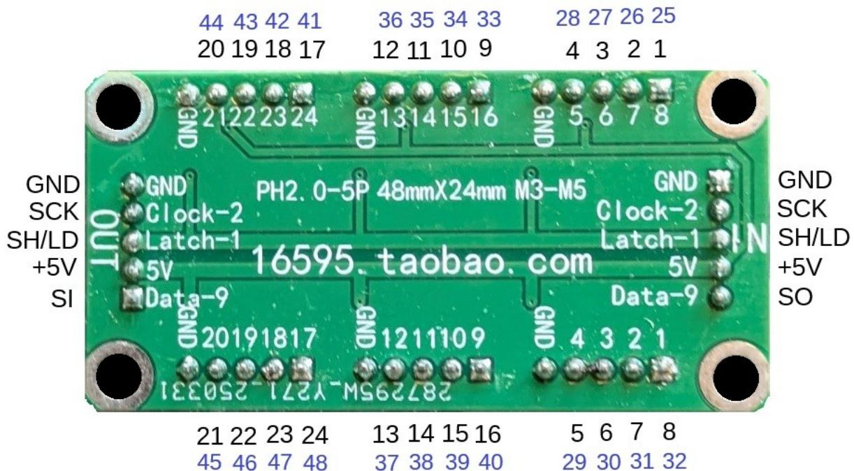
The alternative pin numbering scheme shown above and below the board applies to SPI transfer mode "LSB first". The blue pin numbers apply to a second (higher-order) cascaded board, if any.
